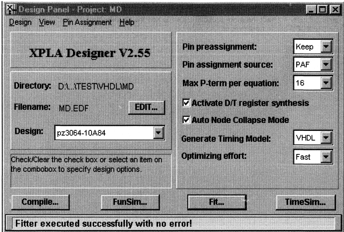
Figure 25: Successful completion of XPLA Designer
